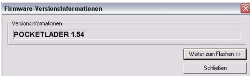
4. Now select whether the new firmware should be downloaded directly from the Orbit server via the Internet, or you want to load a local firmware file (e.g. from a floppy disk).
